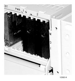
Figure 7. PWR-AVIS With Dual (Redundant) Power Supply Modules
